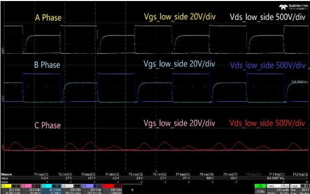
Fig. 9: Vgs and Vds waveform of MOSFETs in full bridge LLC mode
