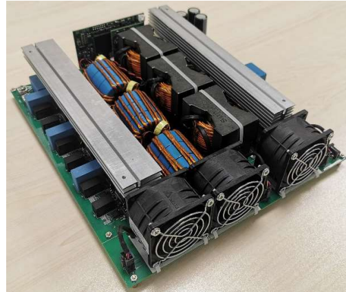
Fig. 6: Photo of the 30kW DC/DC prototype
