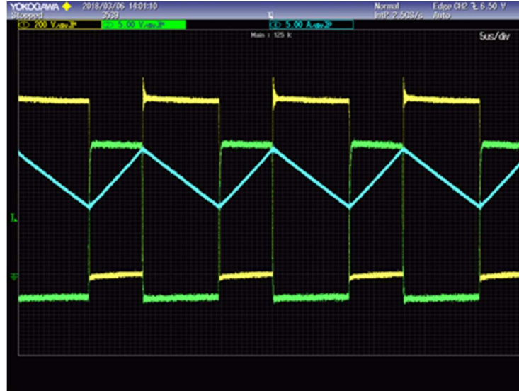
Figure 16. Drain to Source Voltage ( V_{DS} ) (Yellow), Gate to Source Voltage ( V_{GS} ) (Green) and Inductor Current ( I_{INDUTOR} ) (Cyan) Waveforms
