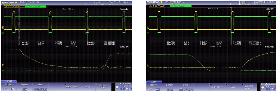
Figure 52. High frequency MOSFET's Gate Voltage (Yellow) and Drain to Source voltage (Green) during turn ON and turn OFF
