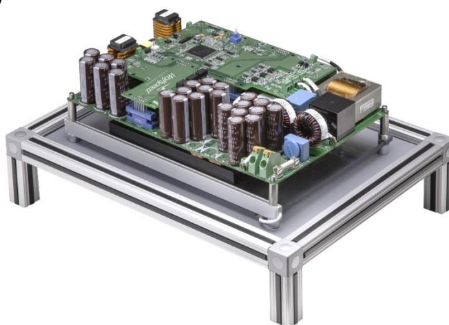
Figure 2. Cree's CRD-06600FF10N, 6.6 kW Bi-Directional EV On-board Charger
