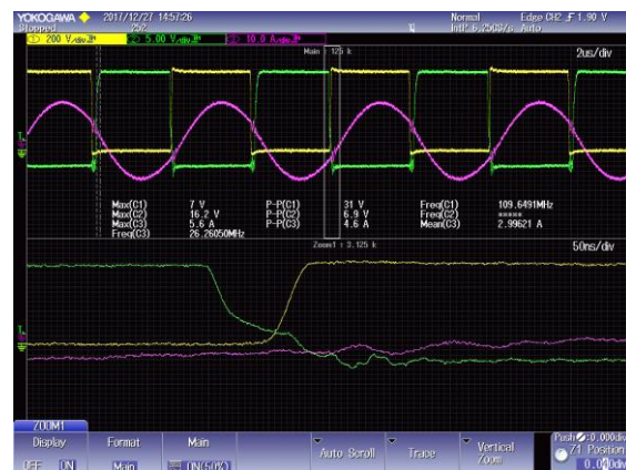
Figure 57. Primary Current (Pink), MOSFET Gate (Green) Voltage and Drain to Source Voltage (Yellow) at 260V and 450V Output
