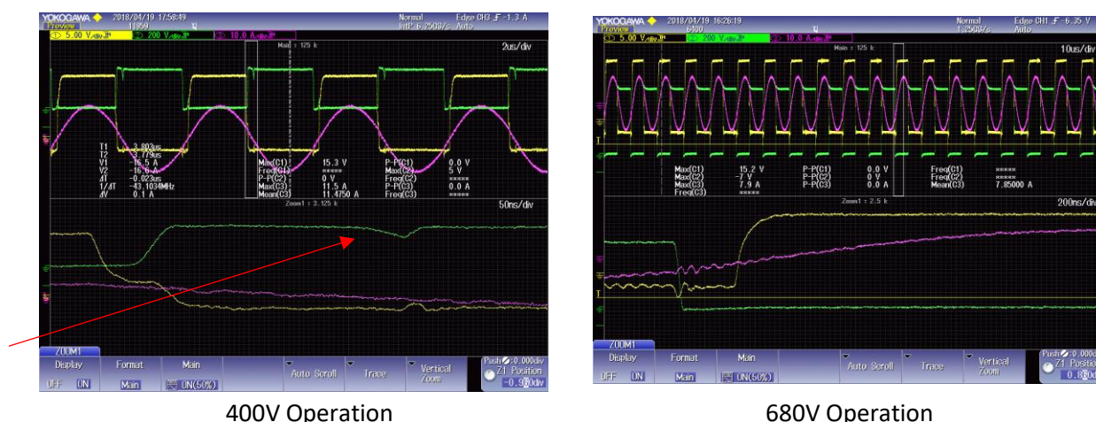
Figure 27. Comparison of ZVS for 400V (Left) and 680V (Right) Operation
