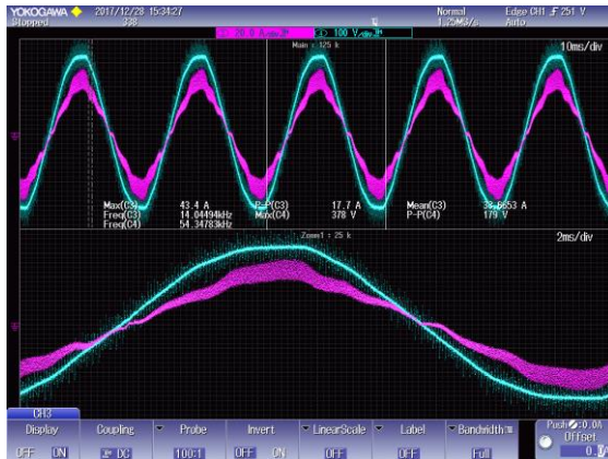
Figure 60. Grid Voltage (Blue) and Current (Pink) Waveforms and Power Analyzer readings for 450V output
