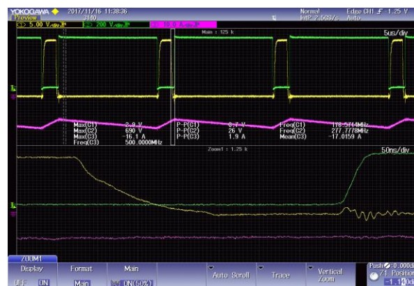
Figure 53. Top and Bottom MOSFET Voltages (Yellow and Green) along with the inductor Current (Pink)
