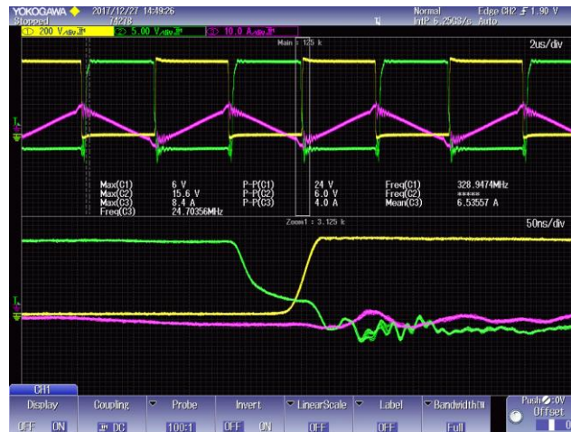
Figure 56. Primary Current (Pink), MOSFET Gate (Green) Voltage and Drain to Source (yellow) Voltage at no load
