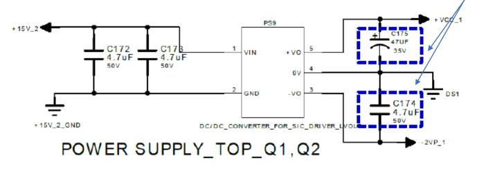
About the capacitor of the output part Aluminum electrolytic capacitor (C175 in the left figure) and laminated chip capacitor (C174 in the left figure) are used.
